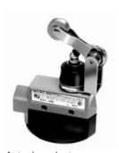
Enclosed Switches Series E6: Top Roller Arm Actuator, One-way, Adjustable with Steel Roller; 1NC 1NO SPDT Snap Action; 0.5 in - 14NPT conduit
